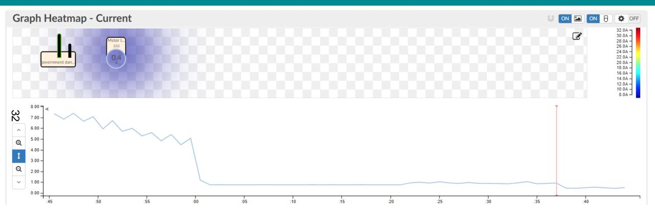
This chart shows the amount of power being used at each home. A clamp is attached to the power supply inside each home, reading are sent back every 5 minutes.
